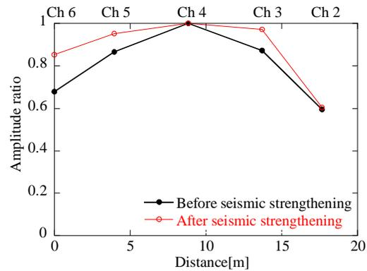
Figure 13. Effect of reinforcement on results of micro-tremor measurements (longitudinal direction).
