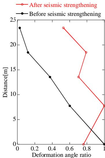
Figure 14. Effect of seismic strengthening on seismic diagnosis (transverse direction).
