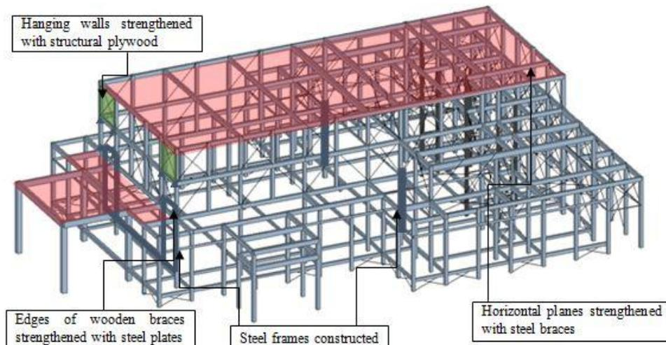
Figure 3. Arrangement of seismic strengthening.
