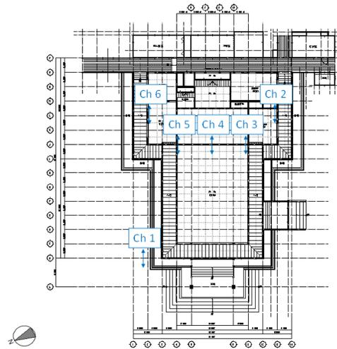
Figure 7. Locations of longitudinal-direction sensors.
