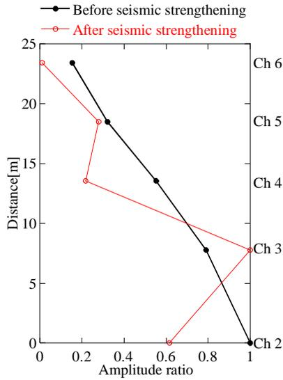
Figure 12. Effect of seismic strengthening on results of micro-tremor measurements (transverse direction).
