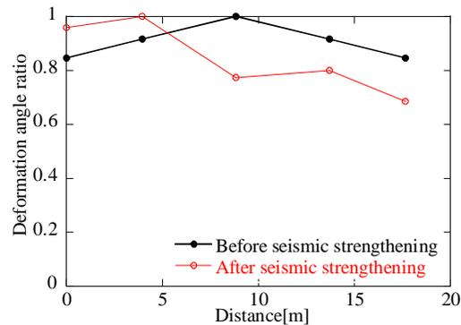
Figure 15. Effect of seismic strengthening on seismic diagnosis (longitudinal direction).
