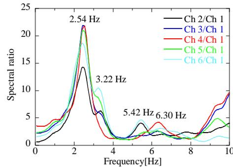
Figure 11. Fourier spectra ratio in longitudinal direction (after seismic strengthening).
