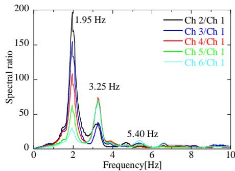
Figure 8. Fourier spectra ratio in transverse direction (before seismic strengthening).
