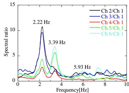
Figure 9. Fourier spectra ratio in transverse direction (after seismic strengthening).
