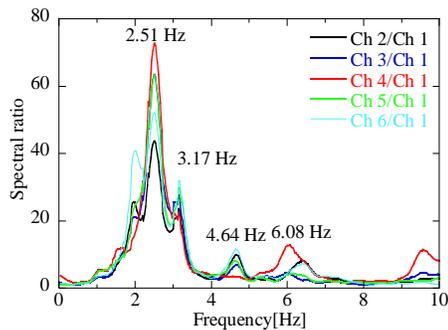
Figure 10. Fourier spectra ratio in longitudinal direction (before seismic strengthening).
