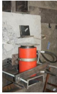
Figure 4. Unilateral shear test loading device.
