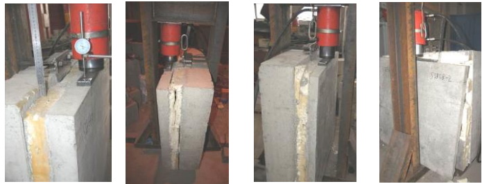
Figure 5. Loading device and destruction diagrams of bilateral-shear test.
