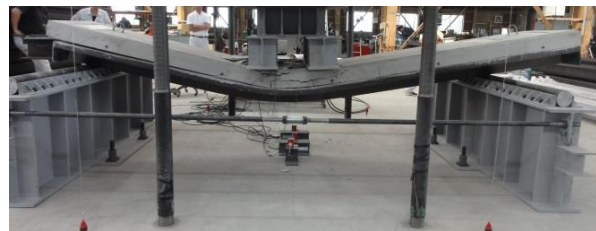
Figure 5. A static loading test (slab).
