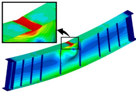
Figure 3. Case 3: 50%-corroded (for combined load).
