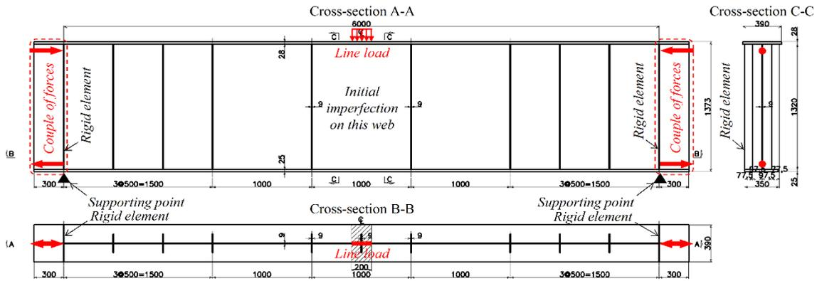
Figure 1. Configurations targeted for analysis and the load conditions.
