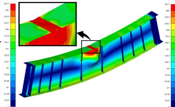
Figure 4. Case 3: 50%-corroded (for pure bending).
