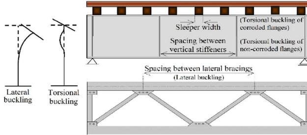
Figure 6. Buckling modes and basic buckling lengths of plate girders.
