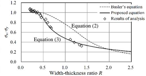
Figure 7. Load bearing capacity curve
