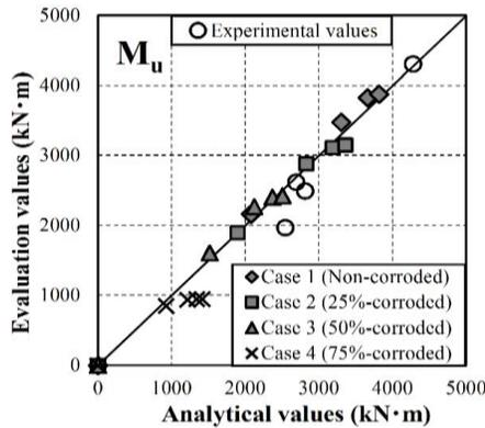
Figure 8. Comparison of analytical and evaluation values (Bending moment  $M_u$ ).
