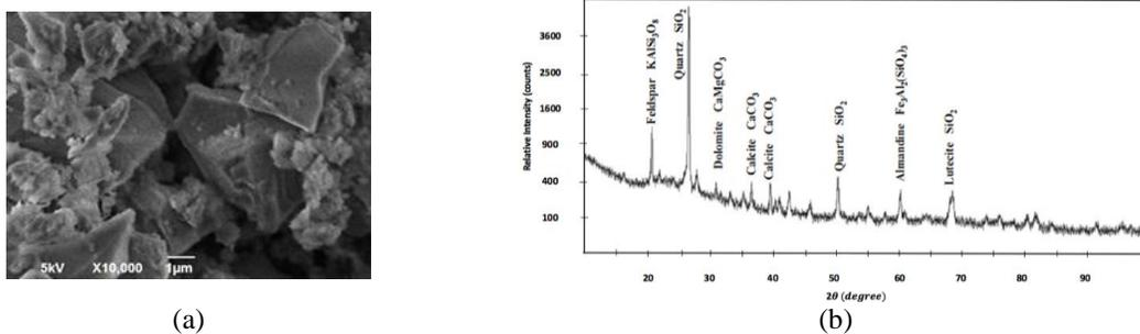
Figure 1. (a) SEM image of CWP particles, (b) XRD spectrograph for CWP.
