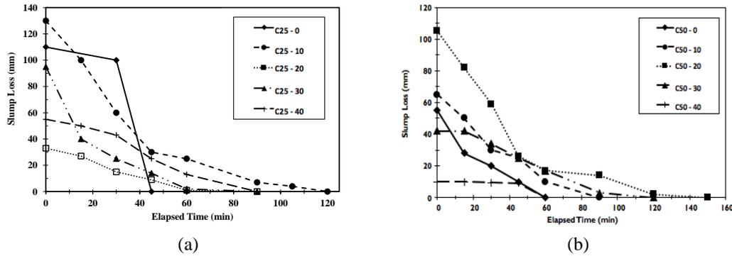
Figure 2. Slump/slump loss results for (a) C25 and (b) C50 mixtures.
