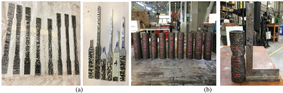
Figure 3. (a) “dog bone” shaped specimens for tensile tests before and after the test; (b) “stub columns” specimens for compressive tests before and after the test.
