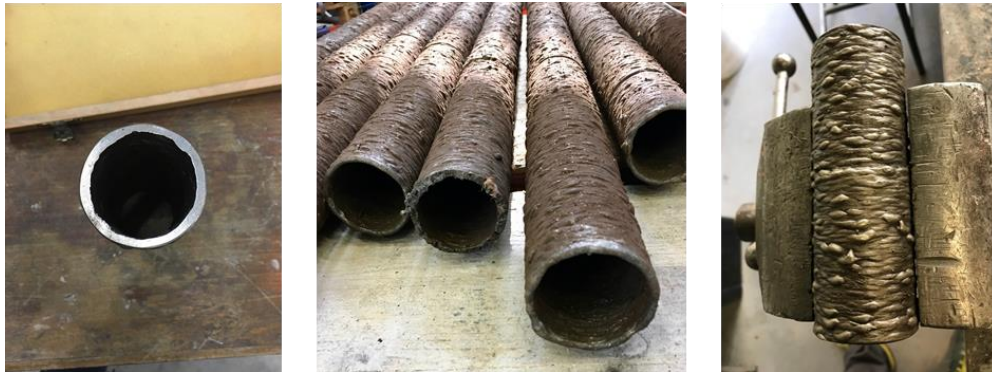
Figure 2. The geometric issue of WAM tubular elements: irregular cross-section, un-straightness, surface roughness.
