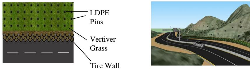
Figure 3. Top view and axonometric view of the proposed slope stabilization.
