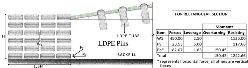
Figure 2. Proposed rectangular tire wall & force calculation.
