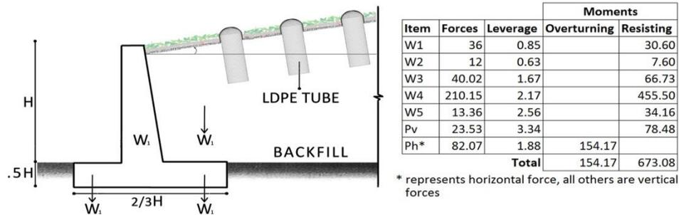
Figure 1. Traditional retaining wall and forces calculation.
