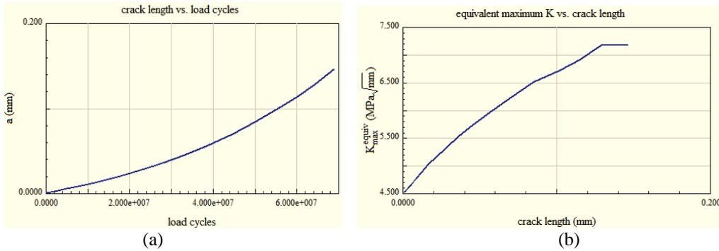
Figure 3. (a) crack growth Vs. number of cycles (b) Crack length Vs.  $K_{max}$ .
