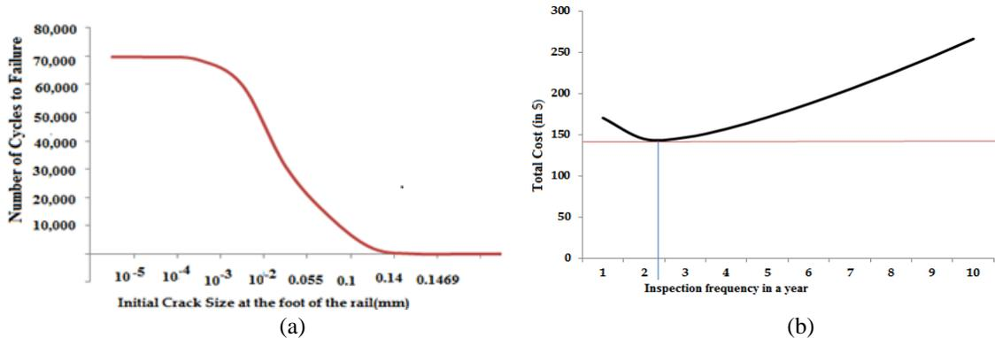
Figure 4. (a) Load frequency and crack growth (b) Total cost (\$) and annual inspection frequency.
