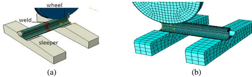
Figure 1. ABAQUS FE Modeling of welded track.
