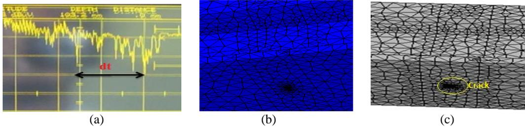
Figure 2. (a) Echograph of UT (b) and (c) Re-meshed Model with elliptical initial crack geometry.
