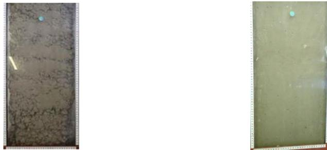
(a) conventional concrete (slump:16.5 cm, air:5.5%). (b) MFC (T15) (S.F.: 47 × 47cm, air: 4.4%).
