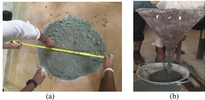
Figure 3. (a) Slump flow test; (b) V funnel test.
