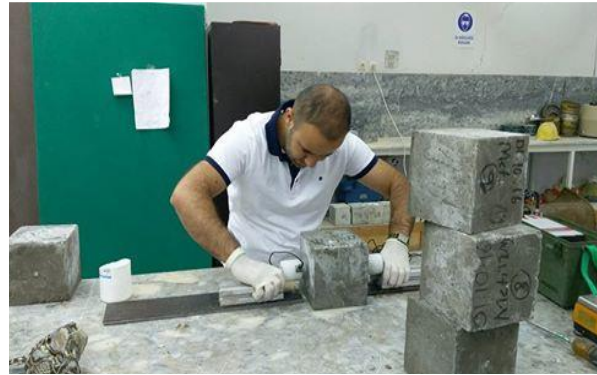
Figure 1. Testing set up of the UPV test.
