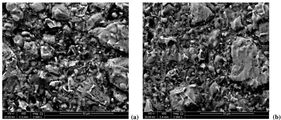
Figure 1. BSE images for (a) freshwater paste and (b) seawater paste at Day 3.
