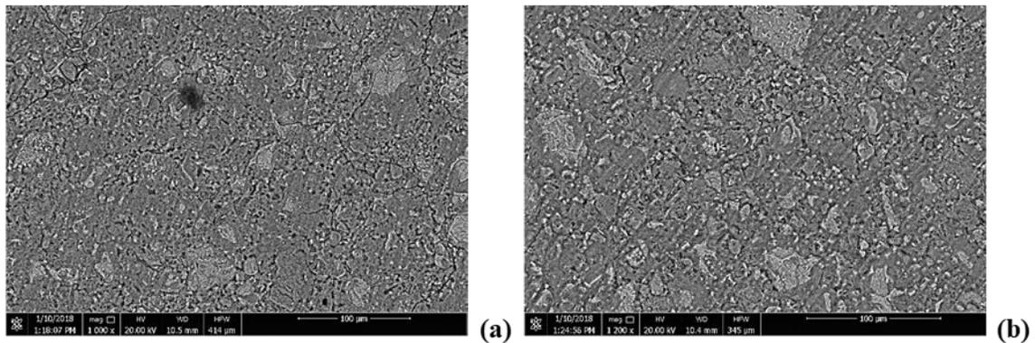
Figure 3. BSE images for (a) freshwater paste and (b) seawater paste at Day 28.
