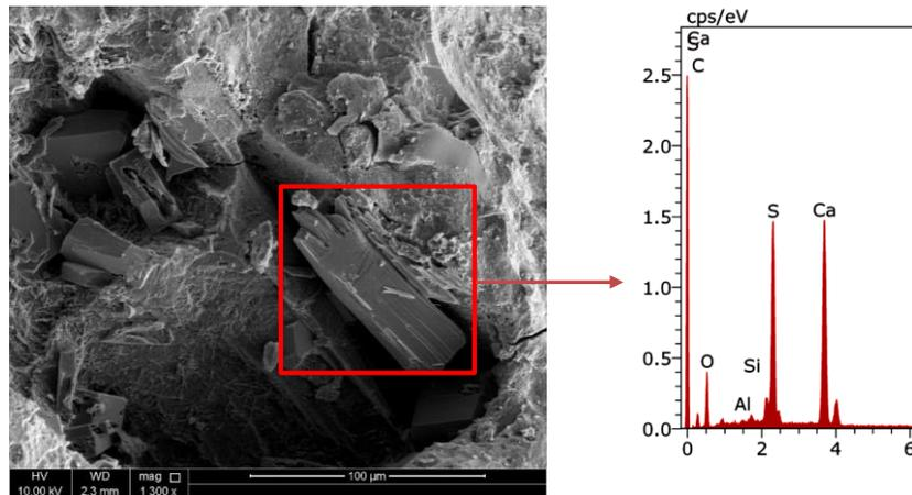
Figure 4. Crystallization of salt impurities in seawater paste.
