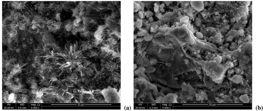
Figure 2. SE images for (a) freshwater paste and (b) seawater paste at Day 3.
