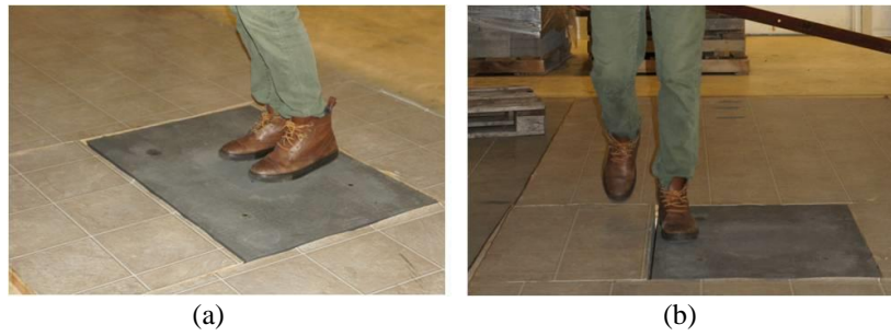
Figure 1. GRF measurement on a flat surface: (a) Weight measurement, (b) Gait measurement.
