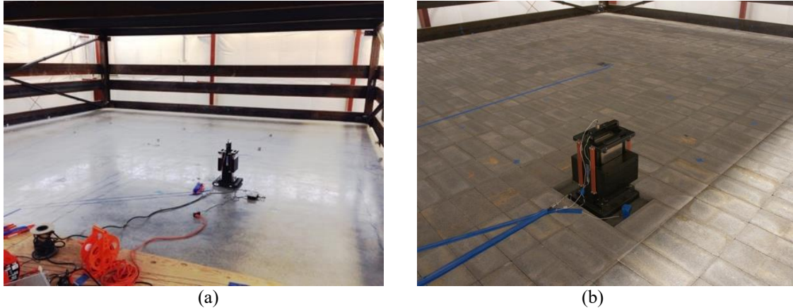
Figure 3. Modal test setups for the floors: (a) Without concrete blocks, (b) With concrete blocks.
