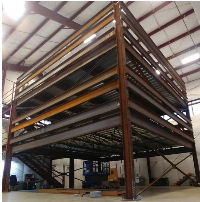
Figure 1. Test structure at the Virginia Tech Vibration Testing Laboratory.
