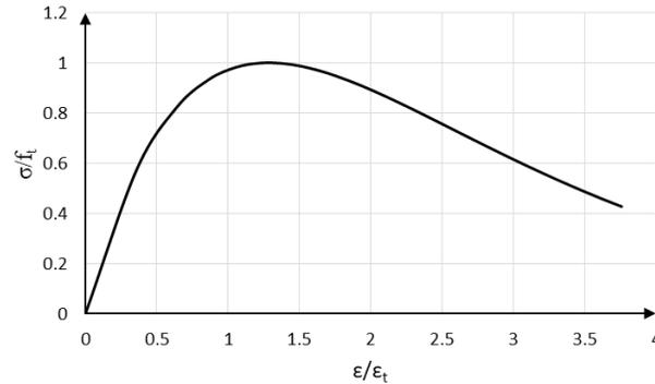
Figure 3. Normalized stress-strain curve of a solid under uniaxial tensile loading.
