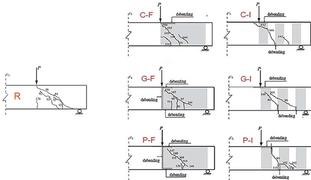
Figure 3. Crack patterns and modes of failure of the tested beams.
