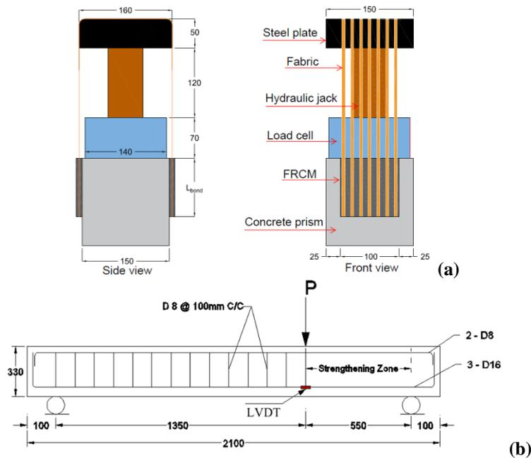
Figure 1. Details for (a) double-shear test specimen, and (b) RC beam specimen.
