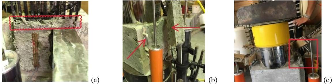
Figure 2. Failure modes – (a) FD in carbon-FRCM; (b) DB in PBO-FRCM; and (c) FR in glass-FRCM.
