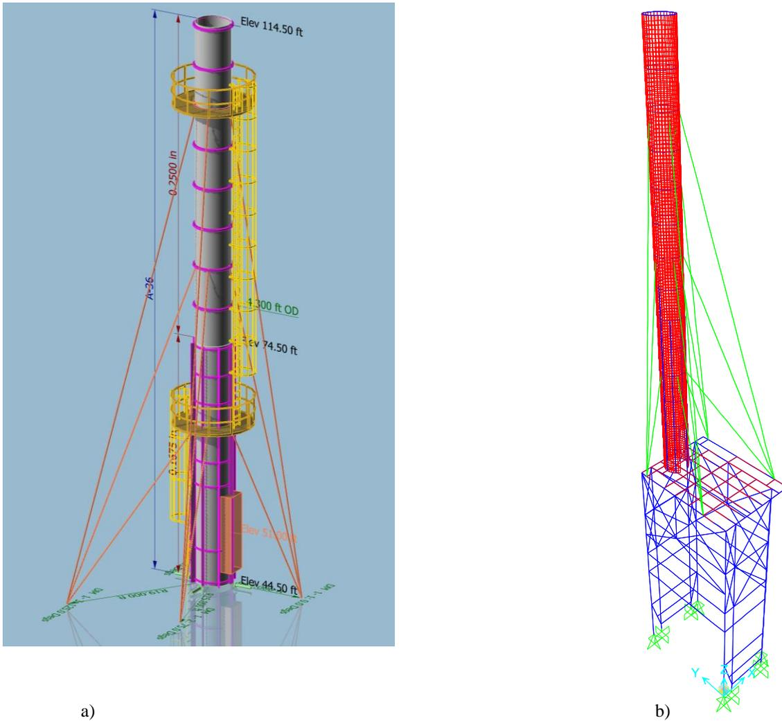
Figure 1. Analysis models: a) Local model with MecaStack; b) Global model with SAP2000 V.20 (2018).
