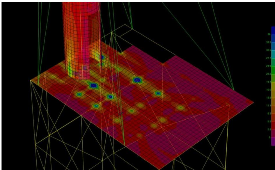
Figure 2. Global model analysis results – computed Von-Mises stress [ksi].
