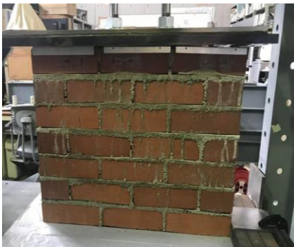
Figure 7. The brick wall specimen without braces.
