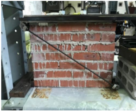
Figure 9. The brick wall specimen with braces.
