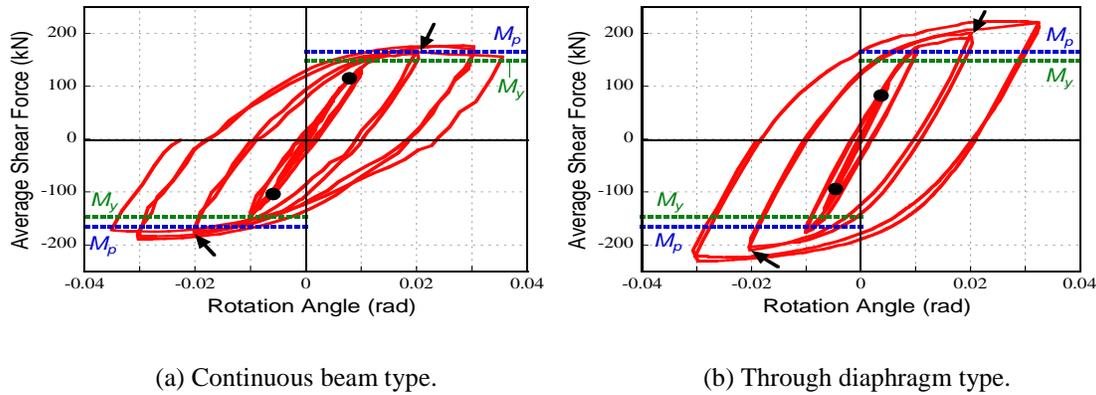
Figure 4. Shear force – rotation angle relation.
