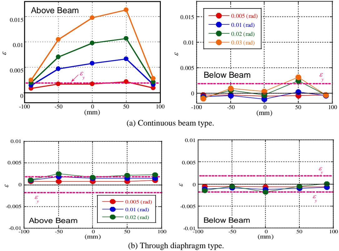
Figure 5. Strain distribution at steel tube flange.
