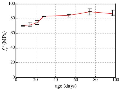
Figure 2. Change of concrete strength.
