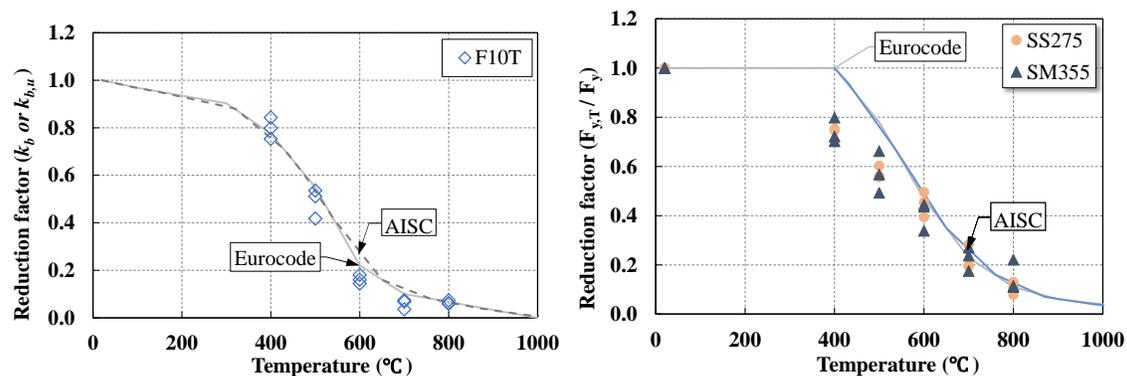
Figure 7. Reduction factor of yield strength compared with existing standards.
