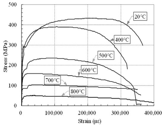
Figure 4. Stress–strain relationship (SS400(SS275)).
