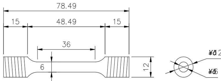
Figure 2. Dimension of tensile test specimen.
