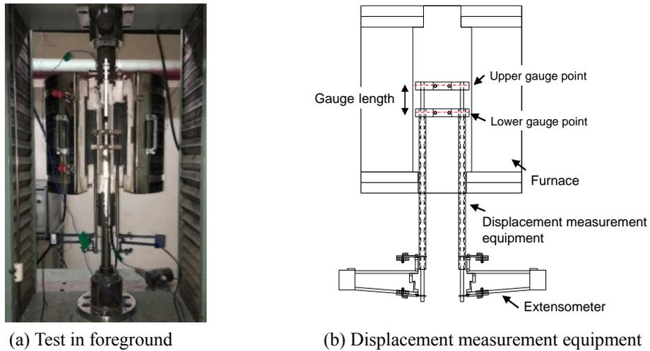
Figure 3. High-temperature tensile test.
