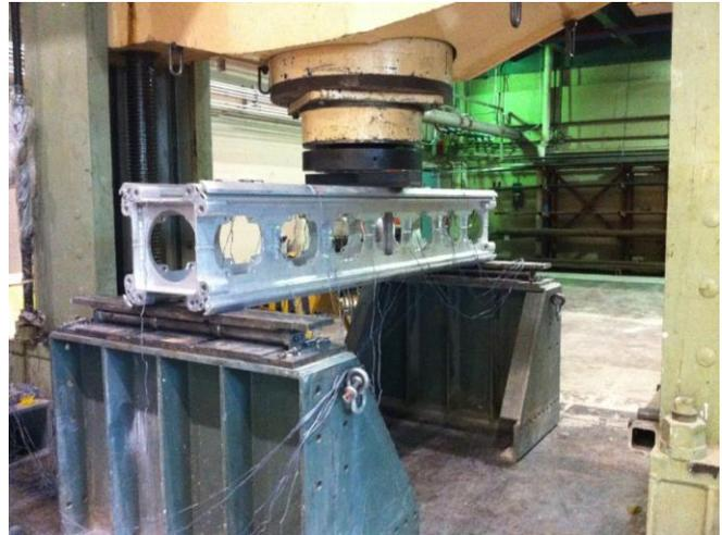
Figure 2. Bending test experimental setup.
