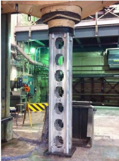
Figure 1. Buckling test experimental setup.
