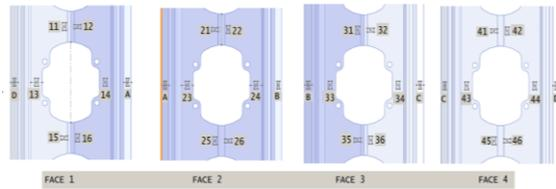
Figure 4. Strain gauge locations for buckling tests.
