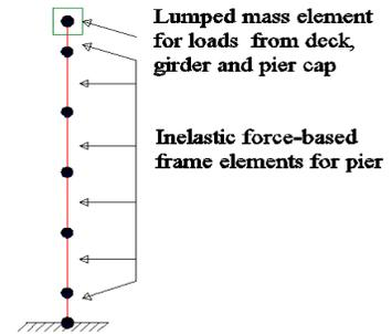
Figure 3. Analytical model of typical pier.
