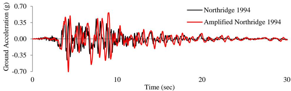
Figure 4. Ground motion accelerations for THA.
