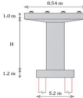
Figure 2. Transverse section of typical Pier.
