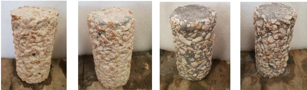
Figure 1. Samples after exposure to sulfuric acid (From left M1, M2, M3 and M4).
