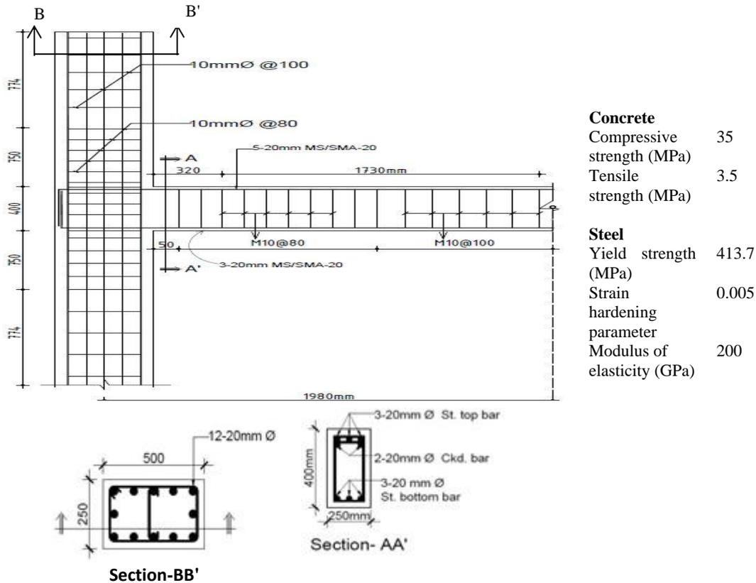
Figure 1. Reinforcement details of beam-column joint and material properties.
