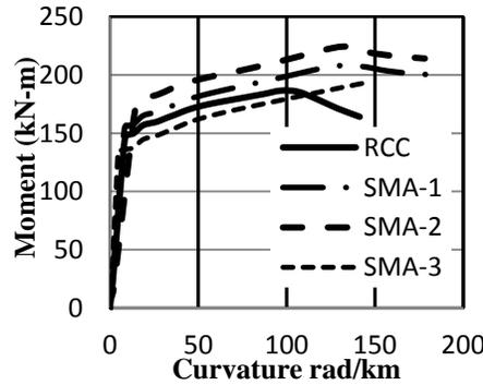
Figure 2. Moment-curvature relationships for steel-RC, SMA-RC-1, SMA-RC-2, SMA-RC-3, beam-column joint.
