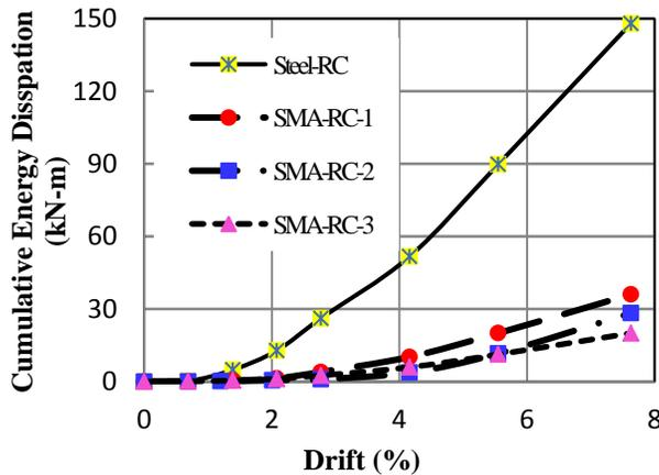
Figure 4. Cumulative energy dissipation-story drift relationships of specimens.
