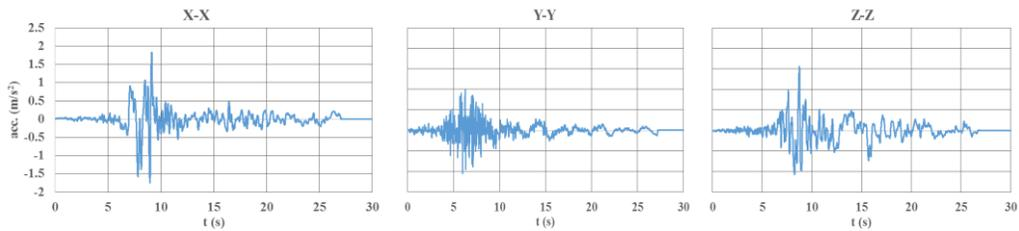
Figure 6. Components of ground acceleration used in the analysis.
