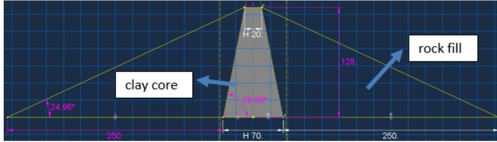
Figure 3. Assumed cross section for the Derbendikhan Dam used in the analysis.
