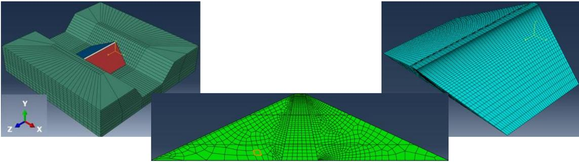
Figure 5. Complete dam assembly with the ground (infinite elements) and meshed dam cross-section and 3D body.
