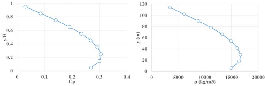
Figure 4. Variation of  $C_p$  Increased mass density due to hydrodynamic effects on downstream slope.
