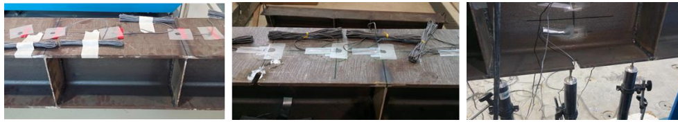
Figure 4. Installation of strain gauges and placement of LVDT's.
