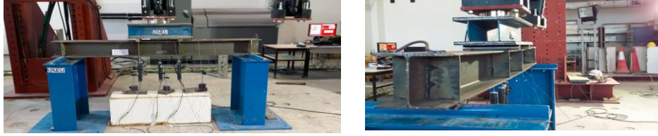
Figure 3. The beams with vertical stiffeners over supports and under loading points.
