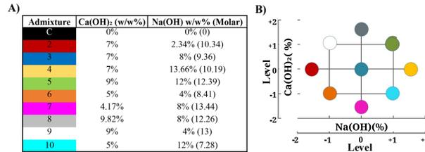
Figure 1. (A) Experimental matrix. (B) Central composite experimental design.
