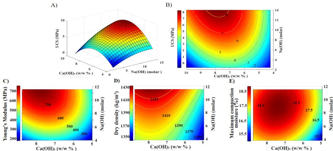
Figure 2. (A) UCS response surface. (B) UCS contour plot. (C) Young’s modulus contour plot. (D) Dry density contour plot. (E) Maximum compaction moisture contour plot.
