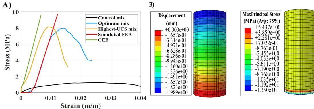
Figure 4. (A) Stress-strain curves. (B) Simulation of displacements and stress distributions for the optimum mix cylinder.
