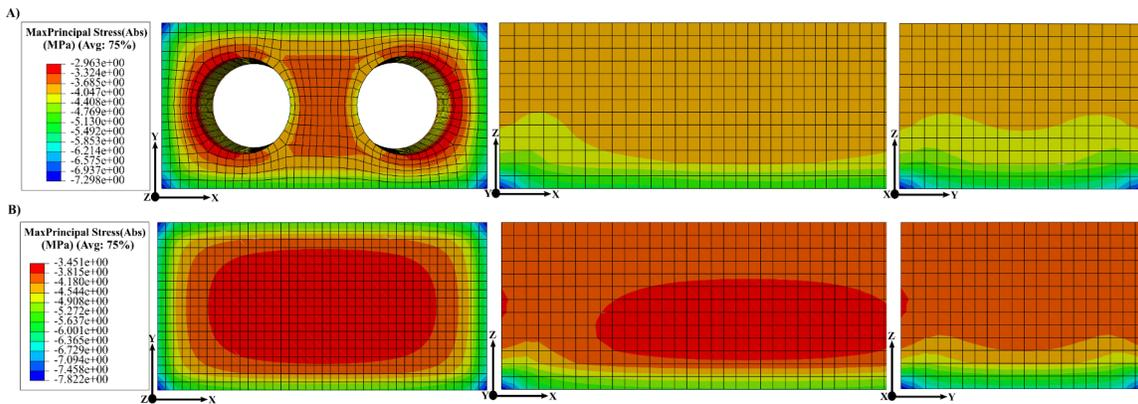
Figure 6. SQS linear response simulation. (A)Hollow block. (B) Solid block.
