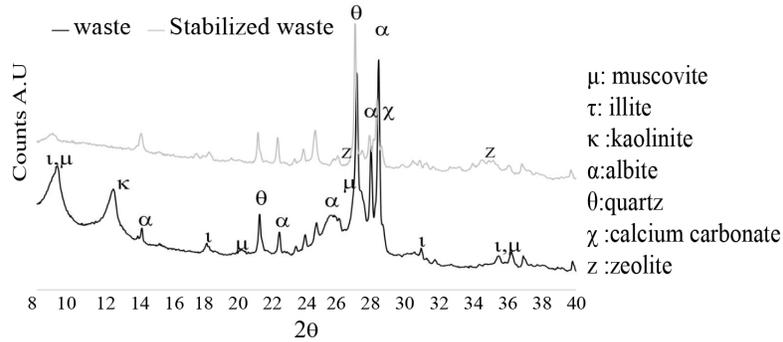
Figure 3. X-ray diffraction of SQS and QS.
